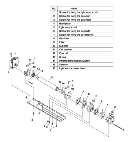
Figure 7-1: Measuring Unit Configuration (Pipe Cell)
